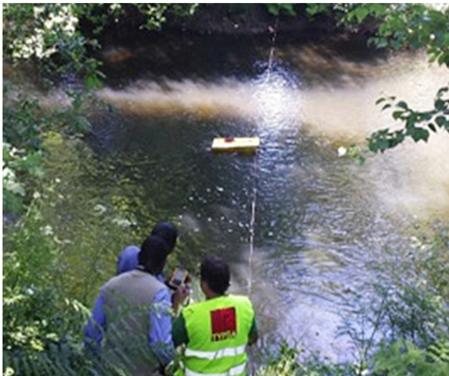
ARA-Norte personnel while performing a direct gauging with the Qliner2 (OTT)
