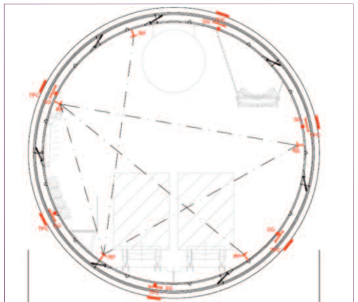
Monitoring of the tunnel ring
