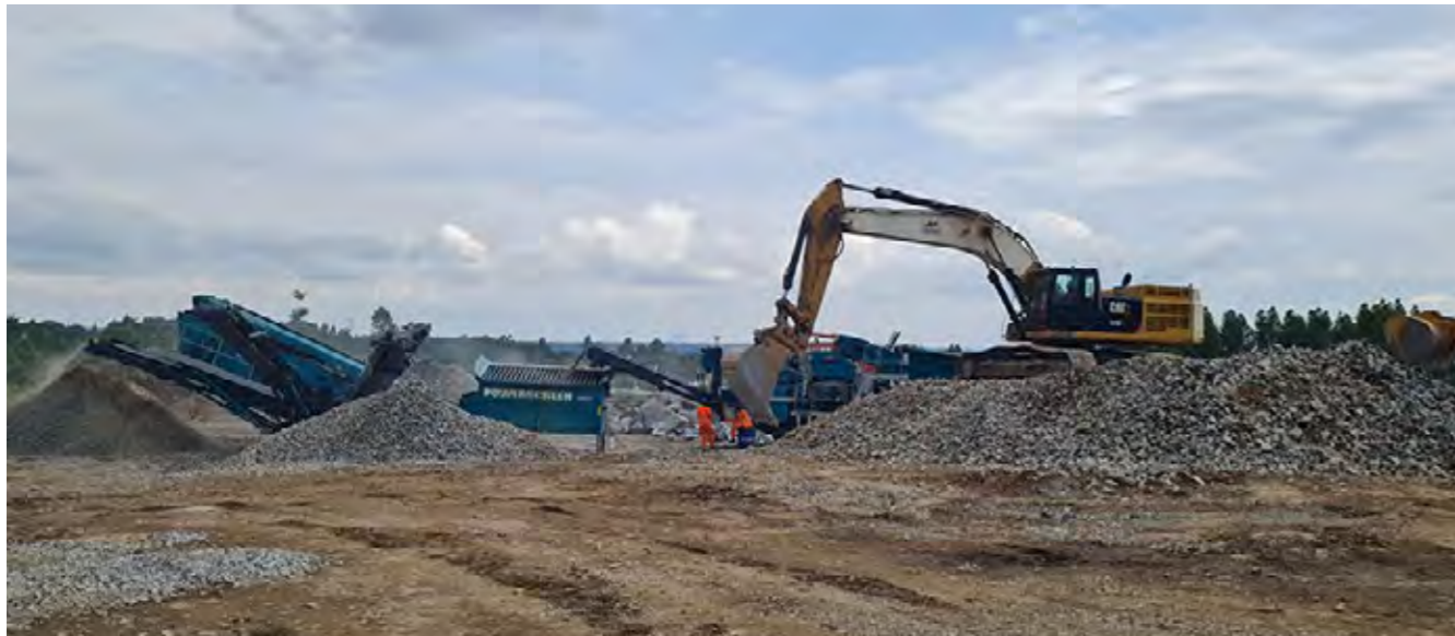
Quarry (crushing plants) – production of rail ballast
